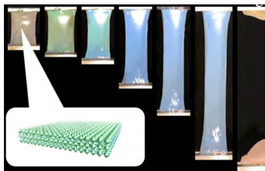
Fig. 1 The photograph of the gel with varied structural color during a stretching test and the schematic structure of the perovskite nanosheet.
