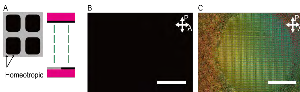
Fig. 1 (A) Schematic illustration of surface modification. (B) A homeotropic texture under no electric field (C) A highly self-organized pattern of defects arrays induced by an electric field obtained by the assist of surface modification. Scale bar, 1 mm.
