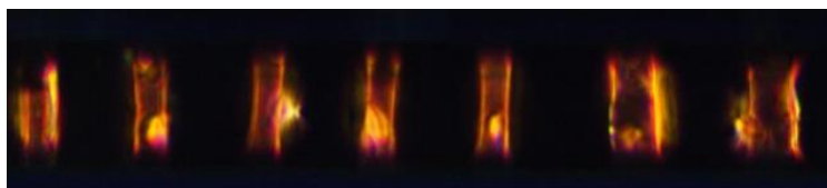
Fig. 1. One dimensional photonic crystal in nematic liquid crystal doped with gold nanoparticles
